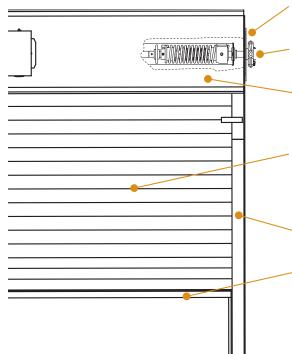
**BRACKETS** - Steel with powder coating to match curtin. Bolt to guide assembly and support counter-balance shaft and curtain.
